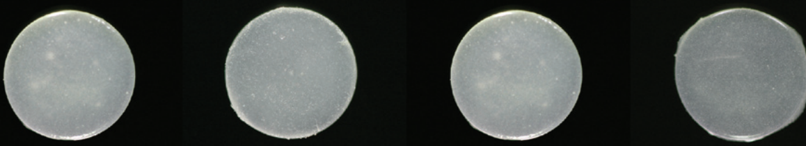
With increasing condensation the translucency of the firing samples enhances. (VINTAGE ZR T-Glass from left to right: without condensation, manual condensation, ultrasonic condensation low, ultrasonic condensation intensive)
